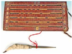
The 'sliding plate' with associated pointed slider was believed to be the predecessor of the Morse keying device described in this chapter.
