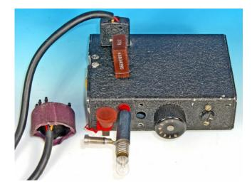
The 'Plug-in transmitter French 1' retrieved its power from a normal broadcast receiver, substituting the AF output valve by a socket and cable. See also Chapter 79.
